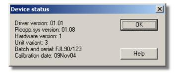
This dialog box displays the details about the ADC status. The calibration date will help you keep track of when the unit should be returned to Pico for annual recalibration (optional).
