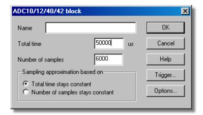
This dialog box only applies to the block method of recording. It is used to select the total time and the number of samples that will be used to take measurements.
