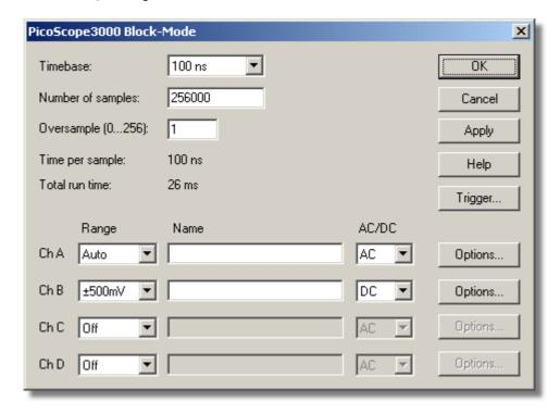
This dialog box is used to select the sampling rate and channels for fast data recording.
