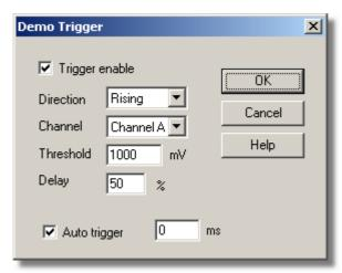
Triggering is used to select the moment at which PicoLog collects data - usually at some fixed time before or after a trigger event.
