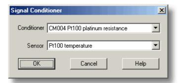
This dialog box provides support for the Pico range of signal conditioners. A signal conditioner provides excitation and/or power for a sensor and then amplifies the output from the sensor.
