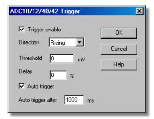
Triggering is used to select the moment at which PicoLog collects data - usually at some fixed time before or after a trigger event.
