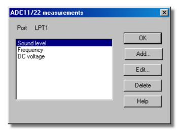
This dialog box is used to build up a list of measurements to measure for a converter. On the left is the current list of measurements and on the right are buttons to update the list.
