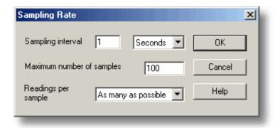
This dialog box sets the sampling rate and defines the action to take at the end of a run.
