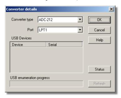
This dialog box is used to specify the details for a converter. Note that it is NOT displayed if you set the **Converter preferences** to automatically select a particular converter.
