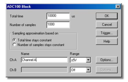
This dialog box only applies to the block method of recording. It is used to select the channels that will be used to take measurements.
