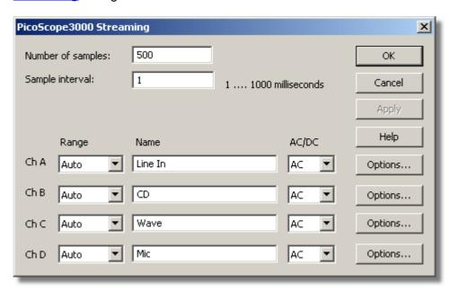
This dialog box is used to select the sampling rate and channels for streaming data recording.
