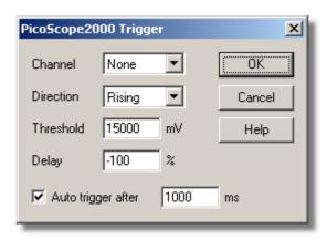
Triggering is used to select the moment at which PicoLog starts collecting data - usually at some fixed time before or after a trigger event.
