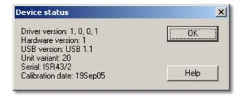
This dialog box displays the details about the ADC connection to the computer.
