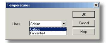
This is used to specify the units for temperature measurements. The options are Fahrenheit or Celsius (Centigrade).
