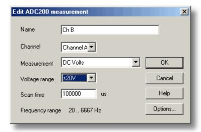
This dialog box is used to enter the details for a measurement.
