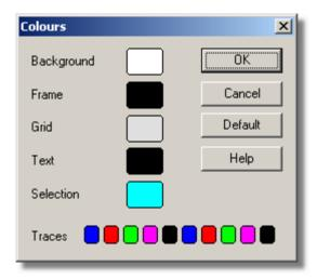
This is used to specify the colours for the background, text and traces for the graph and spreadsheet windows. To change a colour, click on the colour button to open the colour selection dialog box.
