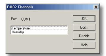
This dialog box is used to select the channels that will be used to take measurements.
