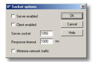
This dialog box is used to specify the details required to establish a link between computers via an IP network.
