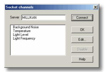
This dialog box is used to establish a connection to another instance of PicoLog running on a remote server computer, and then to select the channels that are to be imported to this instance of PicoLog.
