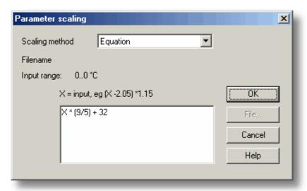
This dialog box is used to specify how to convert a measurement value into some other unit, for example from volts to temperature. It is invoked when you click the Scaling button on the **Parameter options** dialog box.
