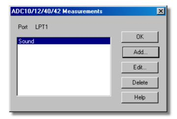
This dialog box is used to build up a list of measurements to measure for a converter. On the left is the current list of measurements and on the right are buttons to update the list.
