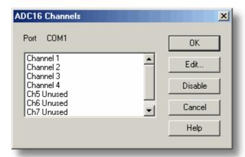
This dialog box is used to select the channels that will be used to take measurements.
